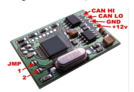
Mode is selectable by applying solder joints – JMP 1 and JMP 2 (see picture).
